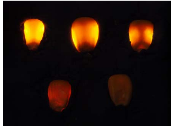
Figure 2. Differing translucence (vitreousness) of corn endosperm types as defined by a light box. Brighter corn endosperms are an index of greater vitreousness and potentially greater prolamin protein concentrations. Corn endosperm types which transmit minimal light are considered opaque.
