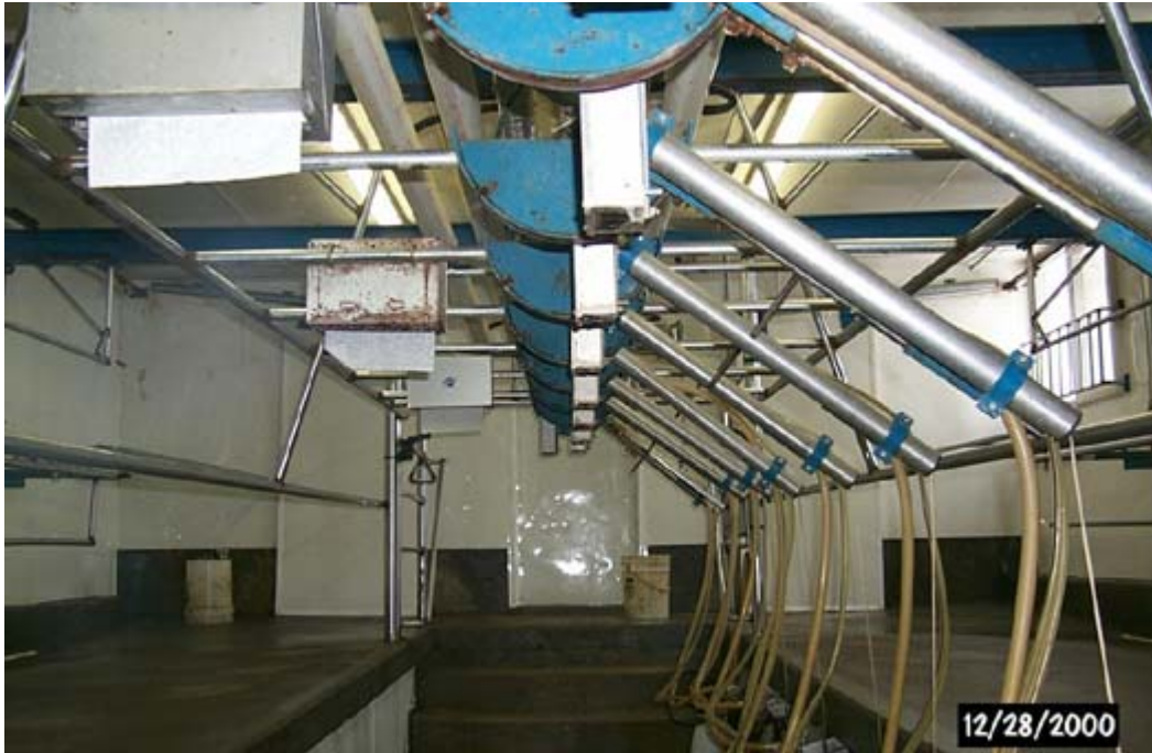
Figure 1. Retrofit parlors have proven to be a low cost way for Wisconsin dairy producers to adopt parlor technology into their operations. This parlor cost was under $34,000.
